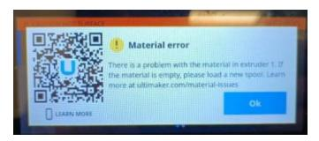
The print head can detect if filament is being properly extruded from the nozzle(s), so the interface will display the error above if no filament is being extruded.
